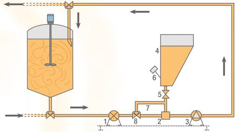
the valve, minimizing aeration. When the powder sensor closes the powder feed valve, product flow can be diverted round a bypass line (7) by the divertor valve (8).
