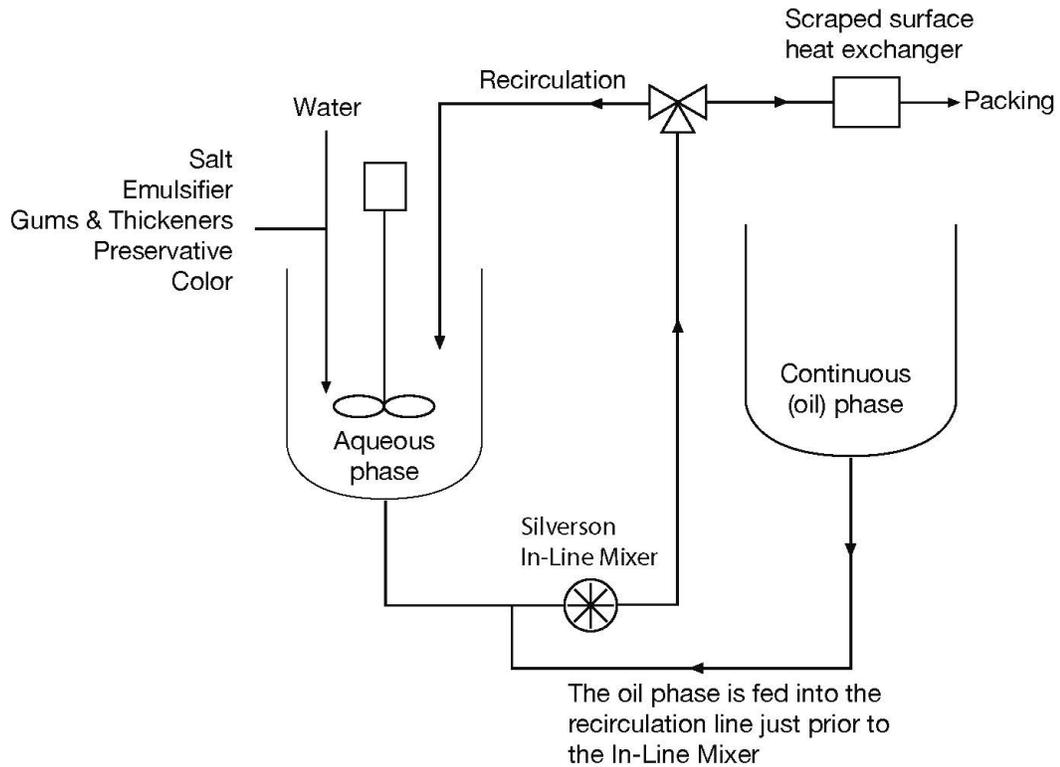
The aqueous phase ingredients are added to the vessel and recirculated through the self-pumping In-Line mixer which disperses and hydrates the materials, rapidly producing a homogeneous agglomerate-free mix.
