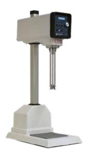
Silverson Laboratory mixers are suitable for the widest range of applications - mixing, emulsifying, homogenizing, disintegrating, and dissolving. With a capacity from 1ml up to 12 liters and the ability to mix in-line with flow rates of up to 20 liters/minute, they offer excellent reproducibility when scaling up and provide an accurate means of forecasting the performance of larger Silverson machines under full-scale working conditions.
